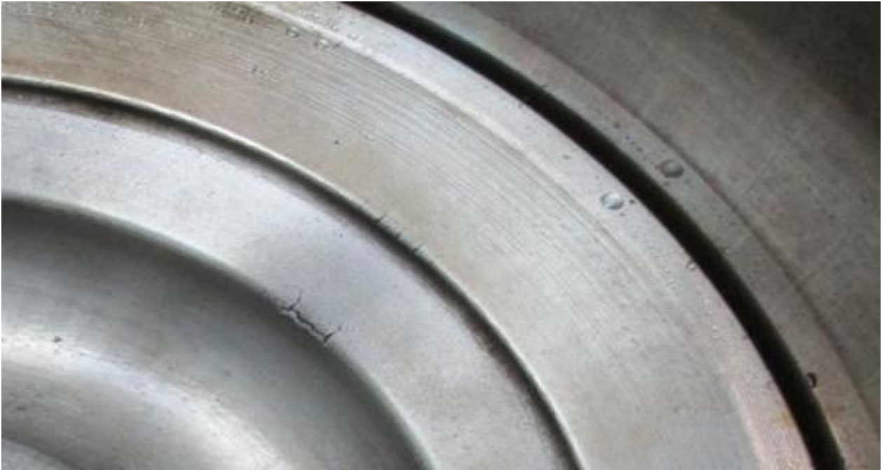
Figure 2.4: CFD piston after the measurement program at CMP
